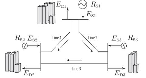
Fig. 2. Texas model: a simplified 3-bus network.
